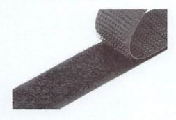
The VELCRO® Brand Loop 001 is a European soft & durable textile loop suitable for the most demanding applications. It is a woven medium profile polyamide loop tape guaranteeing a high cycle life that can be opened thousands of times without losing its strength when paired with the VELCRO® Brand Hook 088.
